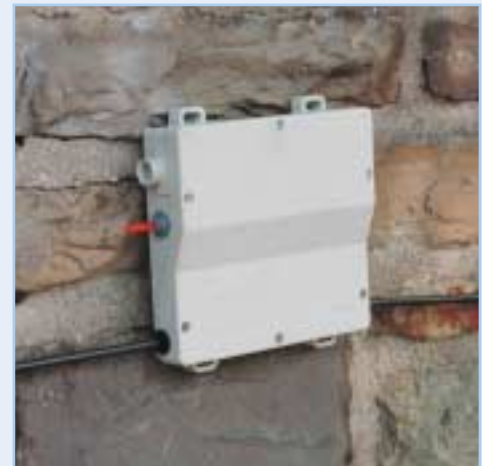
X-Trigger following actuation, visual alarm.
